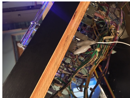
Figure 6 Arduino connection inside of pinball machine
