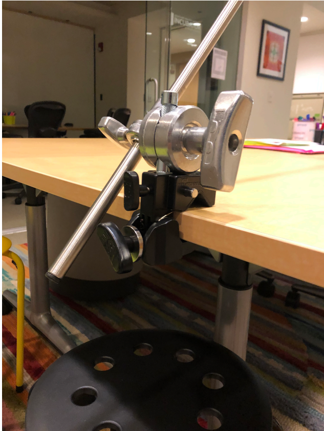
This is a view of the table clamp, this is where the Studio-in-a-Box attaches to the table securely.
