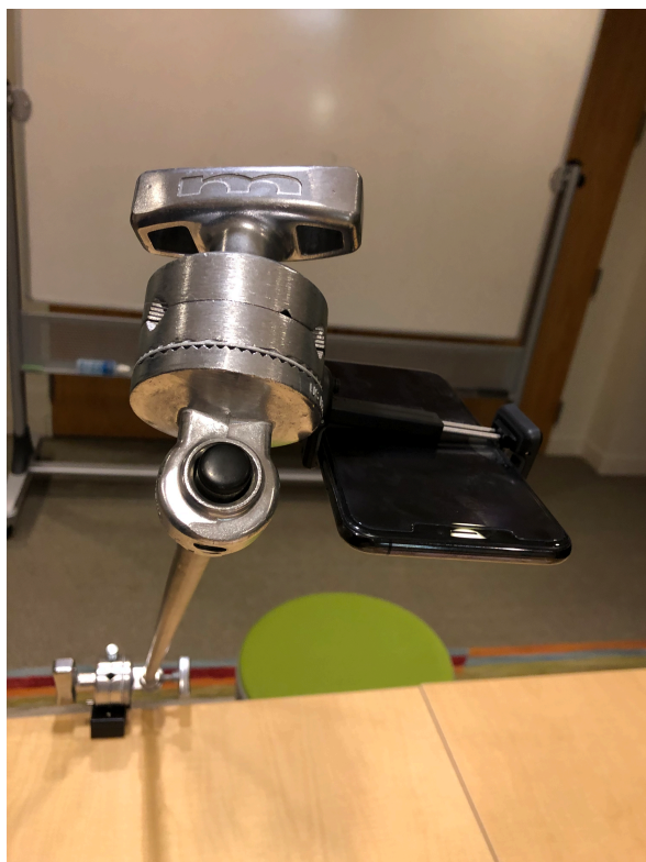
The Phone clamp- this is where the iPhone would attach. For larger or smaller phones/tablets, there would be alternate attachments
