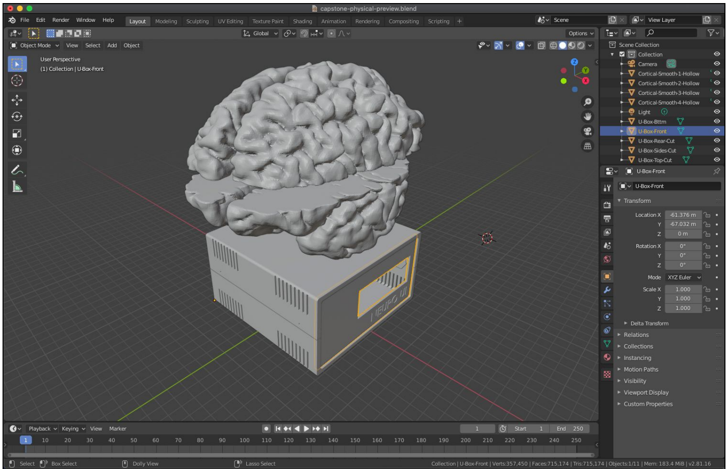
Figure 4: The final STL models for hollowed brain quadrants (eventually printed at half-size for hobbyist-level 3D printer) and microboard enclosure.
