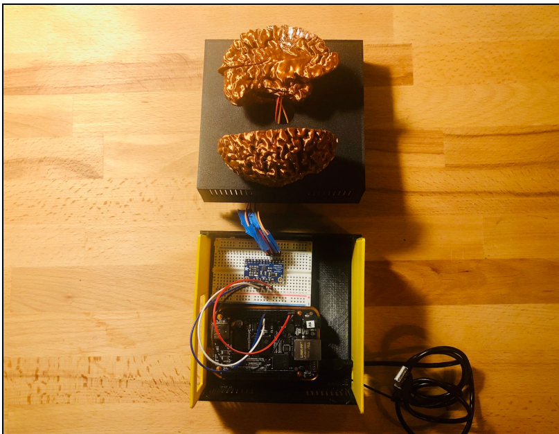
Figure 8: The complete physical UI wired together (the enclosure can be easily opened to access electronics, as seen here).
