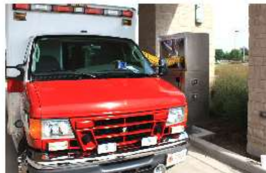
Ambulance hooked up to a MediDock, which provides power and conditioned air. Used with permission of American Idle Reduction, LLC.
