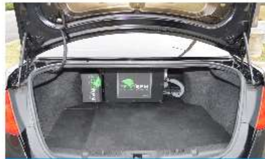
Police vehicle auxiliaries can be powered by a battery pack that fits in the trunk. Used with permission of ZeroRPM, Inc.
